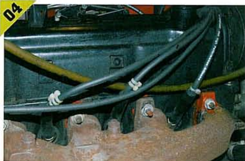
▲ Check the plug leads too. Silicone leads last a long time but do eventually need replacing. Mark the leads so that you don't mix them up if you disconnect them.
