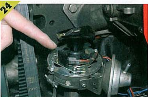
▲ The completed assembly should look similar to this (depending on the distributor being converted). ▼ Check that the wiring clears all the rotating parts. Check this with the vacuum advance unit in both the advanced and retarded positions.
