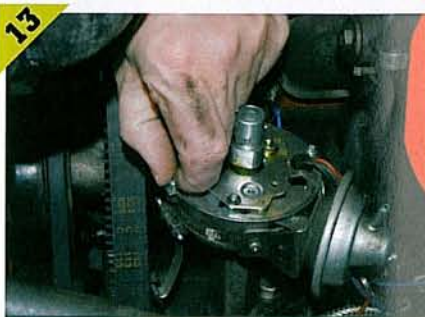
▲ Feed the trigger wires through the grommet. Position them carefully in the back plate then re-fit it to the distributor block. Don't over tighten the screws. ▼ Check that the grommet is positioned correctly and that no wires are trapped or kinked.
