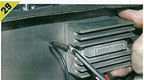
▲ Drill the holes for the fixing screws. Steve recommends titanium coated drills for stainless steel (bought in bulk). ▼ The unit needs a secure earthing point. The stainless body here is perfect, but a GRP body needs a separate earth wire.
