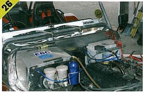
▲ Choose a suitable position for the power module, within reach of the distributor but away from sources of heat. The inner wings or bulkhead are usually suitable. ▼ Hold the module in the chosen position. Mark the positions for the fixing screws.
