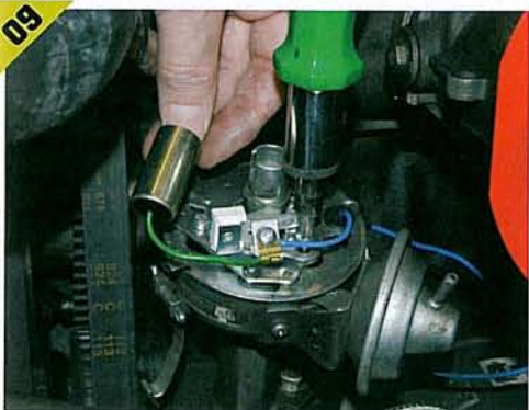
▲ Undo the screw or screws holding the contact breaker points and remove them. ▼ Not essential, but a good time to check the mechanical advance mechanism in the distributor. Remove the screws and any circlips. Lift off the back plate.
