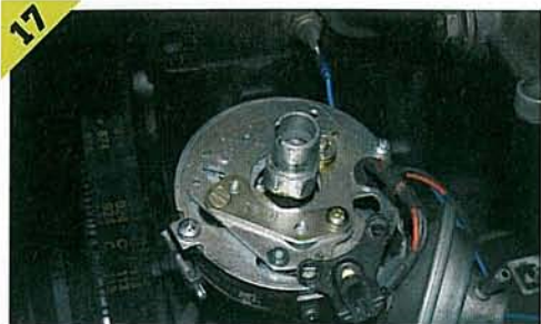
▲ This is the adaptor plate correctly fitted with the trigger ready to go on.
