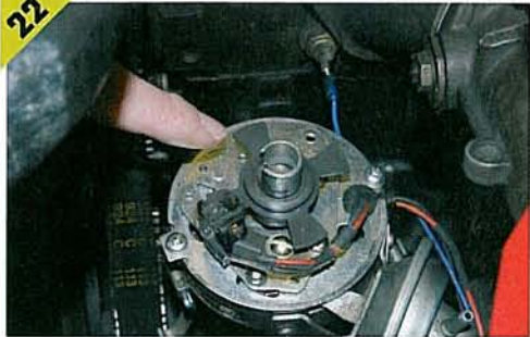
▲ This shows the chopper in position. The blades should pass approximately mid way between the two lenses.
