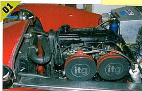
▲ Excellent access to the distributor in this car. In extreme cases it may be easier to remove the distributor from the car.
