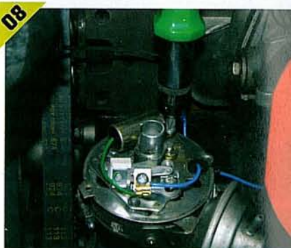
▲ A typical points and condenser set up. In this distributor the wire exits through a special grommet. You have to lift the plate slightly to remove it.
