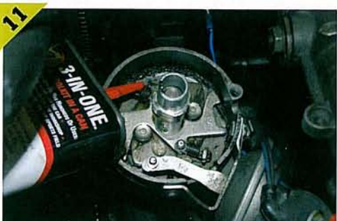
▲ Check that the bob weights move freely and put a drop of oil on the pivots and spring retaining posts. ▼ Left to right: The power module, the trigger fitting kit, the optical trigger and the 'chopper'.
