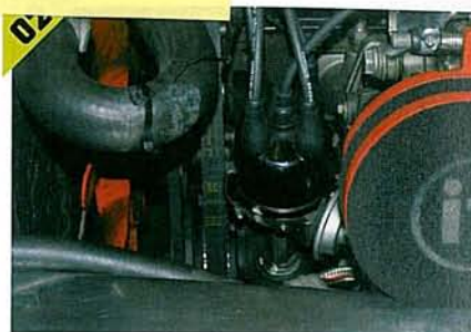
▲ If you need to remove it, mark it and the engine block with Tipp-Ex so that it can be refitted without altering the timing.
