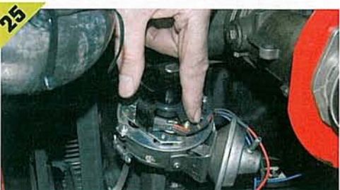
▲ The completed assembly should look similar to this (depending on the distributor being converted). ▼ Check that the wiring clears all the rotating parts. Check this with the vacuum advance unit in both the advanced and retarded positions.
