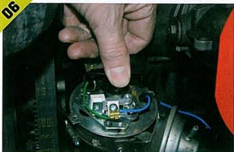
▲ Lift off the rotor arm. Check the contacts for wear and pitting. Once again, replace it if there is the slightest doubt. ▶ Check for side play on the distributor shaft. A small amount of wear is acceptable with contactless ignition, but too much means the distributor needs replacing. ▶▶ Undo the securing screw and remove the condenser.
