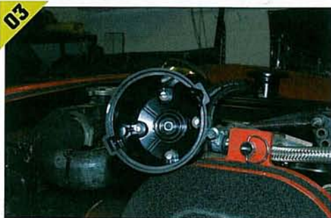
▲ Check the distributor cap for cracks, pitted contacts, erosion or signs of tracking. Replace it if there is any doubt.
