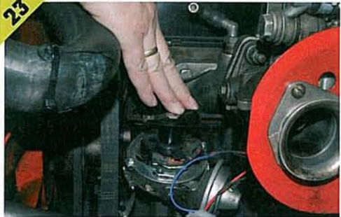
▲ Replace the rotor arm. Locate it correctly on its keyway. It sits on top of the chopper unit.
