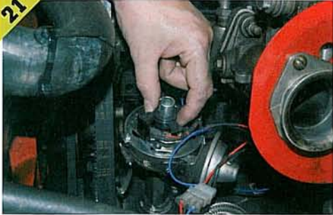
▲ If necessary, turn the engine over so that the chopper blades clear the trigger unit when it slides into place. Push it fully on until it stops.
