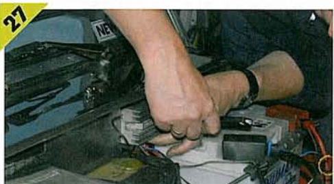
▲ Choose a suitable position for the power module, within reach of the distributor but away from sources of heat. The inner wings or bulkhead are usually suitable. ▼ Hold the module in the chosen position. Mark the positions for the fixing screws.
