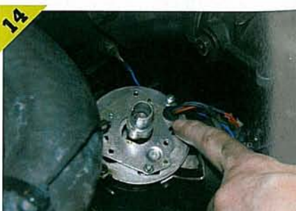
▲ Feed the trigger wires through the grommet. Position them carefully in the back plate then re-fit it to the distributor block. Don't over tighten the screws. ▼ Check that the grommet is positioned correctly and that no wires are trapped or kinked.
