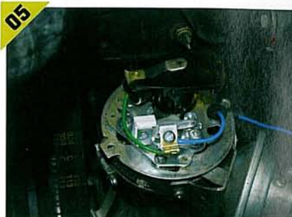
▲ A typical points and condenser set up. In this distributor the wire exits through a special grommet. You have to lift the plate slightly to remove it.
