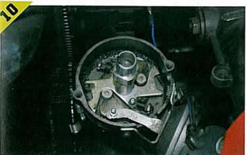
▲ Undo the screw or screws holding the contact breaker points and remove them. ▼ Not essential, but a good time to check the mechanical advance mechanism in the distributor. Remove the screws and any circlips. Lift off the back plate.
