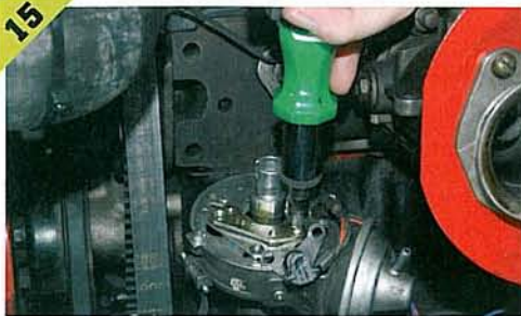
▲ Using the screws supplied in the fitting kit, fit the adaptor plate to the distributor.
