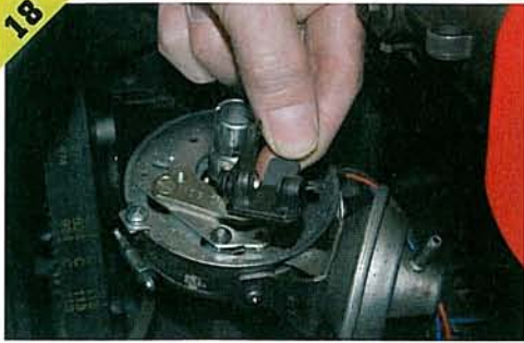
▲ The lenses can be seen here. One emits UV light. The other detects it. Avoid touching the lenses if possible.
