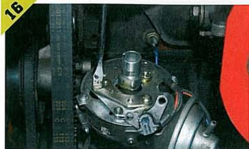
▲ Special countersunk screw. The trigger fits over it so it has to be flush.
